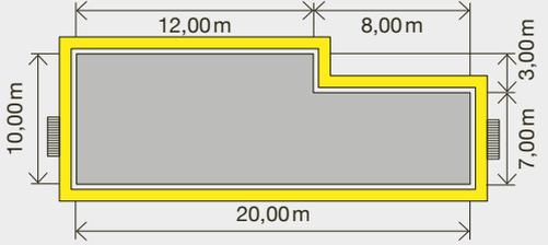
$$A = 60,00 \text{ m} : 50 \text{ m}/\text{accesso} = 1,20 > 1 = 2 \text{ accessi verticali}$$
